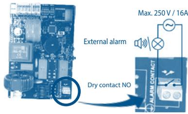
Option of externalising the alarm signal. Dry contact (no voltage) NO (normally open) operated by a relay.
